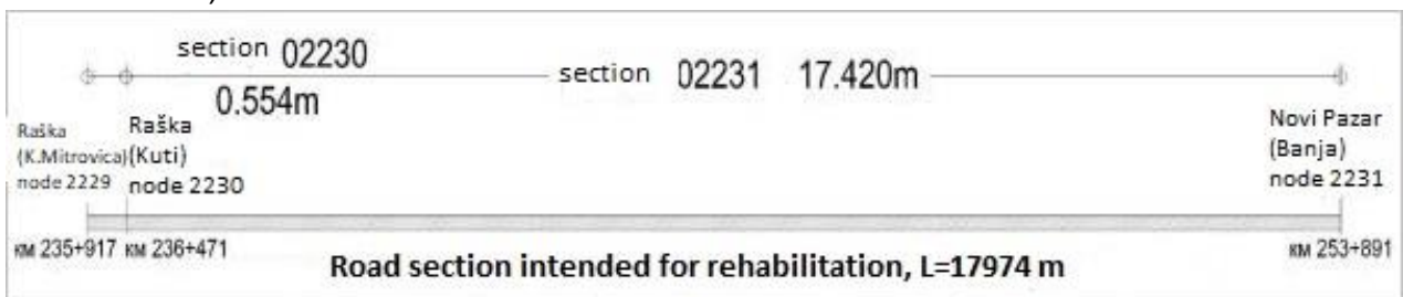
Figure 3. The length of the road section intended for rehabilitation (heavy maintenance)
