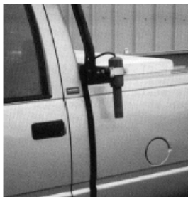
Truck-mounted infrared thermometer
