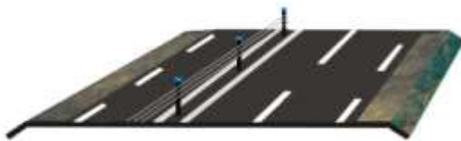
Separation with median barrier
