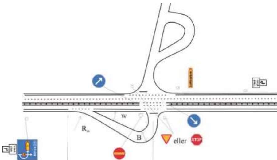
Typical design of a connection of an access road with left turn possibilities
