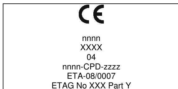
Figure 2.5.6.8: CE mark for expansion joints according to ETAG032-1
