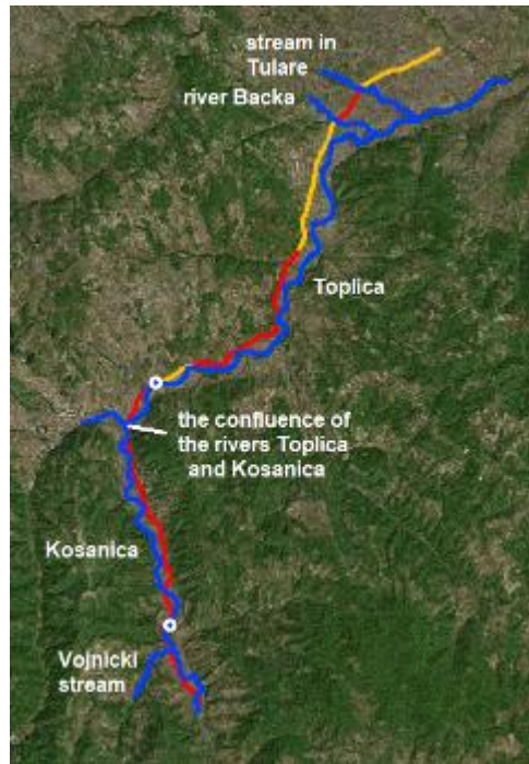
Figure 25. Watercourses intercepted by the section Beloljin - Kursumlija - Rudare There are eight bridges on the route foreseen for rehabilitation, although two bridges (the bridge over the Backa River and the bridge over the archaeological site) are located on the part of the section where no heavy maintenance is foreseen.
