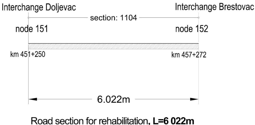
Figure 1.2: Scheme of the road foreseen for rehabilitation (heavy maintenance)
