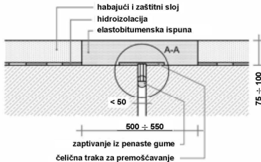
Figure 13 Detail of the asphalt expansion joint
